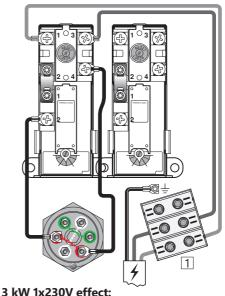
Wire from the right thermostat to the element is removed. The jumpers on the element are removed as shown and wires from the left thermostat is fitted as shown. One of three heating pipes are in use.
